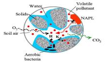
Figure 2: Conceptual model for a VOC biodegradtion in unsaturated porous media
