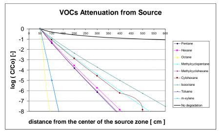
Figure 3: Gas-phase concentration of the VOC. Concentrations are divided by the initial concentration of the source zone.
